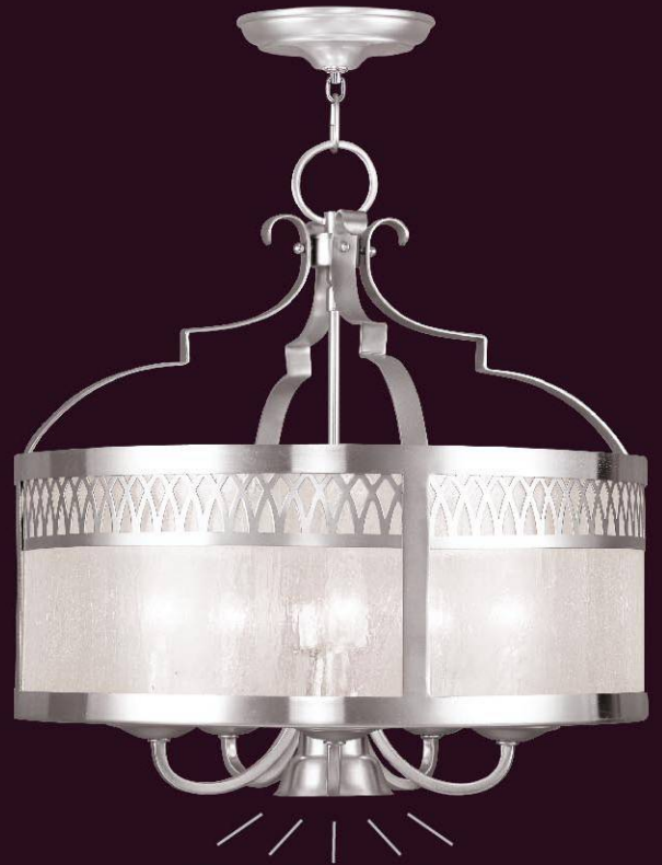
4735-91 Chandelier 20" Dia x 20" H Chain 3', Wire 10', Canopy 6" D Max Watt: 5 x 60 Cand Base + 1 x 50 W R20 Downlight Uplight / Downlight 3-Way Switch Included.
